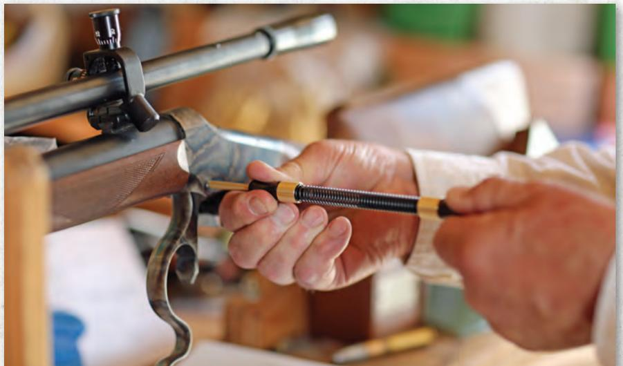
*The Wyoming Sight Drifter makes removing the lever pivot pin on a Low Wall Winchester rifle a breeze.*
