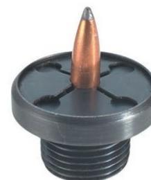
The Forster instructions state that, “To prevent damage to your puller, be sure the mouth of the case only lightly contacts the underside of the puller's spring steel jaws”, and “CAUTION — Do not run your case
