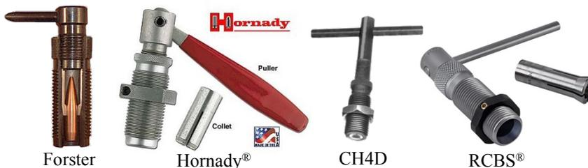
To use a collet bullet puller, raise the ram so the bullet enters the collet, clamp the collet onto the bullet, and then lower the ram. The bullet remains in the collet. When the collet is released, the bullet simply drops out the bottom of the die and into your hand.
